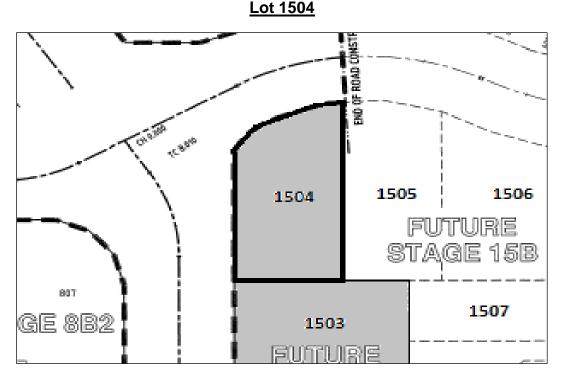
Approximate lateral extent and maximum depth of controlled filling to 1.0m. Level 1 Certification is limited to within this area.
