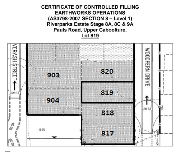
Approximate lateral extent and maximum depth of controlled filling to 0.5m. Level 1 Certification is limited to within this area.
