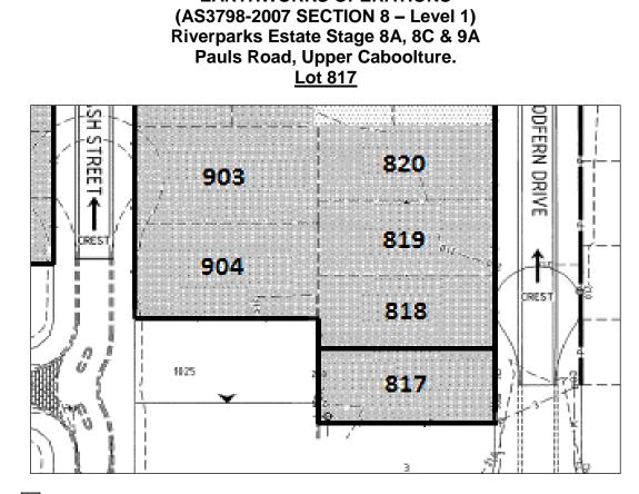
Approximate lateral extent and maximum depth of controlled filling to 0.6m. Level 1 Certification is limited to within this area.
