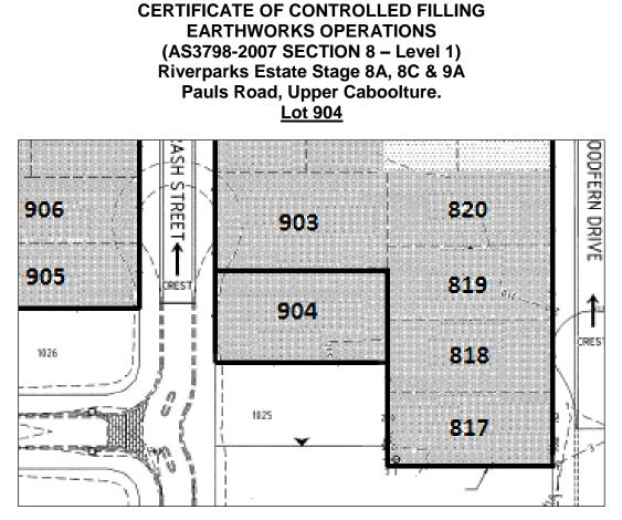
Approximate lateral extent and maximum depth of controlled filling to 0.6m. Level 1 Certification is limited to within this area.
