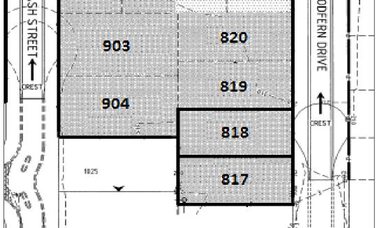
Approximate lateral extent and maximum depth of controlled filling to 0.6m. Level 1 Certification is limited to within this area.
