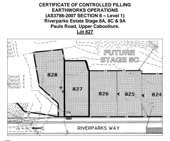
Approximate lateral extent and maximum depth of controlled filling to 1.5m. Level 1 Certification is limited to within this area.
