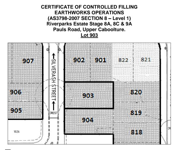
Approximate lateral extent and maximum depth of controlled filling to 0.6m. Level 1 Certification is limited to within this area.
