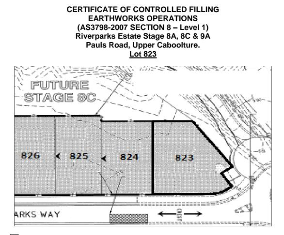
Approximate lateral extent and maximum depth of controlled filling to 2.0m. Level 1 Certification is limited to within this area.
