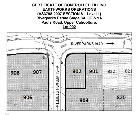
Approximate lateral extent and maximum depth of controlled filling to 0.4m. Level 1 Certification is limited to within this area.
