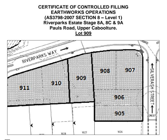
Approximate lateral extent and maximum depth of controlled filling to 0.3m. Level 1 Certification is limited to within this area.
