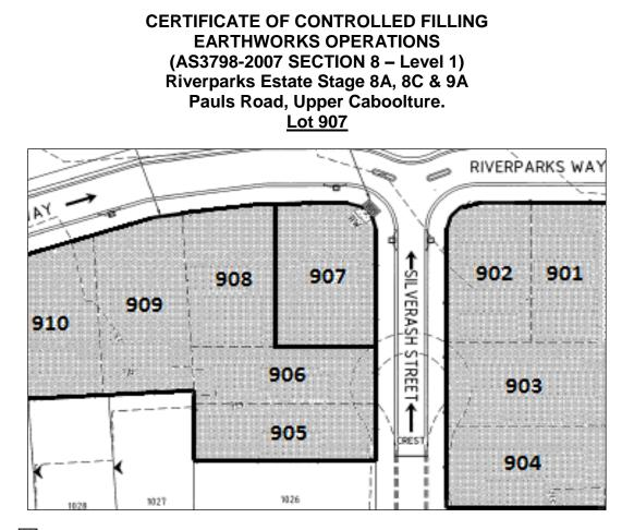
Approximate lateral extent and maximum depth of controlled filling to 0.3m. Level 1 Certification is limited to within this area.
