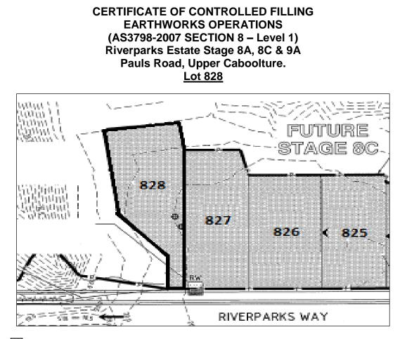
Approximate lateral extent and maximum depth of controlled filling to 1.8m. Level 1 Certification is limited to within this area.
